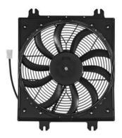
To prevent damage if a cooling fan gets blocked, the circuit powering the fan needs a time-delay type fuse with the correct amperage rating. This installation uses 1x suction fan - part number FAN0606 (F27P-12E8004-41S). The nominal running current is 7 amps.
